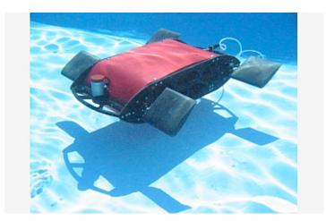
Madeleine, a biologically inspired underwater robot, is helping scientists and engineers better understand the most energy-efficient way to use flippers for locomotion.
