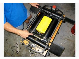
Madeleine's swim skin comes off after a dip. The oscillation of each flipper can be controlled independently to test the impact of different gaits on her motion.
