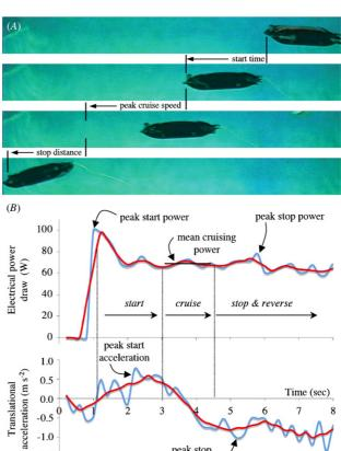
Figure 3. Experimental response variables. Sample data from a four-flippered trial, gait  $[(0, \pi), (0, \pi)]$ , with a peak cruising speed of 0.71 m s<sup>-1</sup>. (A) Kinematic variables measured from an underwater video. (B) Power draw and translational acceleration from on-board sensors. Acceleration corrected for gravitational acceleration. Blue lines are raw data; red lines are low-pass filtered. Raw data used for measurements.
