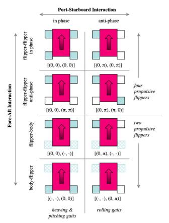
phase matrix = [(front left, front right), (rear left, rear right)] where  $\pi$  is 180° out of phase ("anti-phase") with 0 and where (-,-) indicates fins present but not propulsive.
