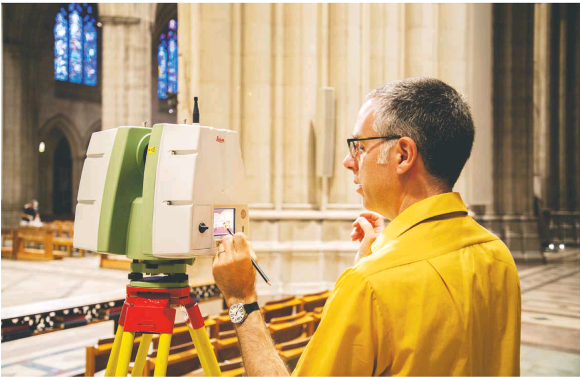
Andrew Tallon scans the Washington National Cathedral using a Leica laser scanner. An expert in Gothic architecture, Tallon discovered that many of Europe's historic cathedrals harbored small deviations from perfect vertical and horizontal lines.
